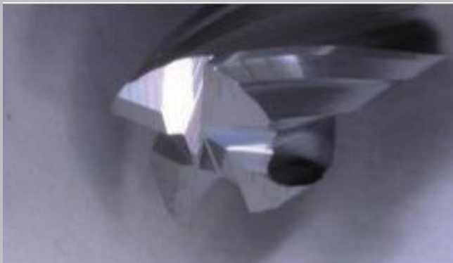
Observation of the end tip of a \Phi 10 End mill at 20x magnification.
